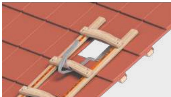
Typical use of safety hook, model Z (pos. 1)
